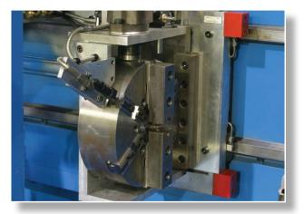
Servo-driven hitchfeeder has quick-change jaws for shaped tubes. Use a full-range jaw set for cutting round tubes.
