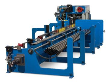
For high-volume cutting of round tubes, our strap-type or chain-type bundle loaders handle large bundles for continuous production.
