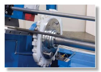
Servo-driven dials rotate to position for each tube shape. Single tubes are transferred into the cutoff machine.
