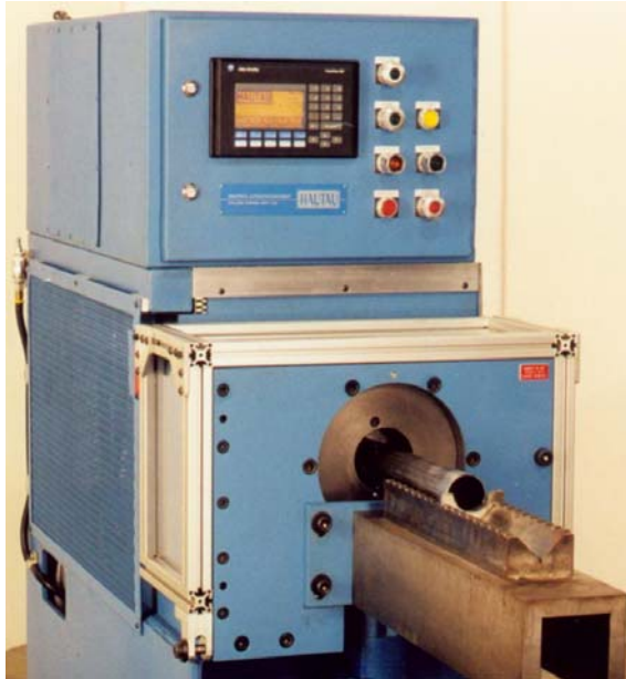
C30S with Servo Tool Feed
